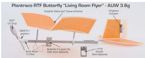
Fig. 2.6 Butterfly 3.6 Gram Living Room Flyer All Up Weight is Less than a sheet of typing paper!
